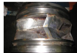
Impeller after cleaning.
