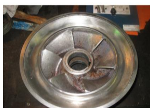
Impeller after cleaning
